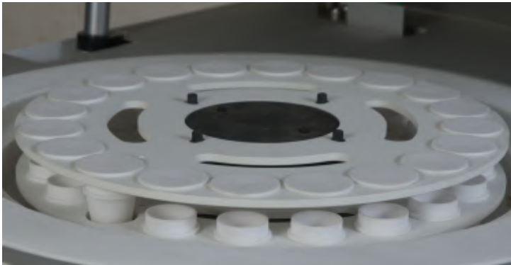
Weighing with crucible lids open
