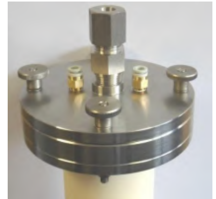
Triple flange end seal with thermocouple gland
